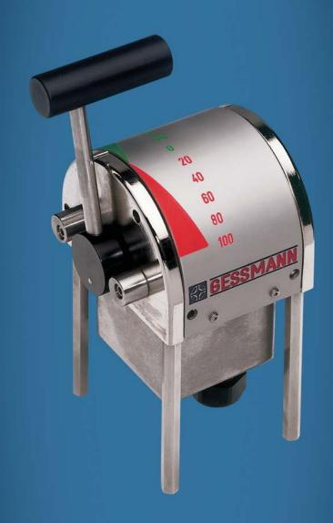
The single-axis controller S3 is a rugged switching device according IEC/EN 60947-5-1 for nautical navigation applications. The modular design enables the switching device to be used universally. The S3 is resistant to oil, maritime climate, ozone and UV radiation.
